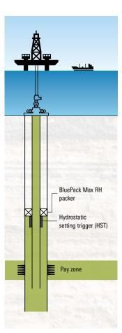
High-pressure retrievable hydrostatic-set production packer in a deepwater one-trip completion.
