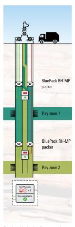
Retrievable hydraulic-set, multiport production packers in a multizone intelligent completion on land.
