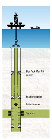
High-pressure retrievable hydraulic-set production packer in a deepwater gravel-pack completion.
