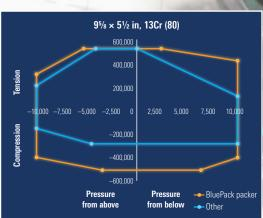
Operating envelopes for the 7-in × 3½-in (left) and 9%-in × 5½-in (right) BluePack Max RH\* high-pressure retrievable hydraulic-set production packers compared with conventional packers. Packer bodies are made of 4140 and 13Cr steel, respectively, with yield strength of 80,000 psi.
