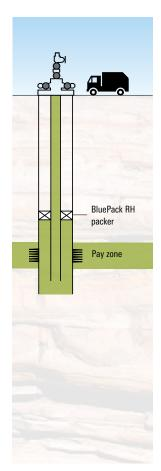
Retrievable hydraulic-set production packer in a single-zone completion on land.
