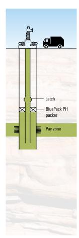
Permanent hydraulic-set production packer in a single-zone completion on land.
