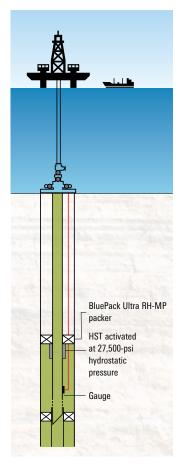
Ultrahigh-pressure retrievable hydrostatic-set, multiport production packer in very deep water.
