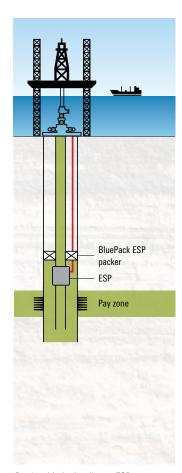
Retrievable hydraulic-set ESP production packer in a single-zone offshore completion.
