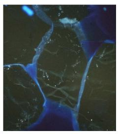
Fluid inclusions in UV light on the boundary of various mineral grains provide a unique chemical signal in the FIS analysis conducted in the PetroFecta analysis workflow.
