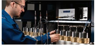
*Core analysis, such as measurement of the electrical properties of formation samples, provides important information to tune log interpretations.*
