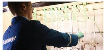
Careful core cleaning techniques are performed using a Dean-Stark apparatus to determine water content.
