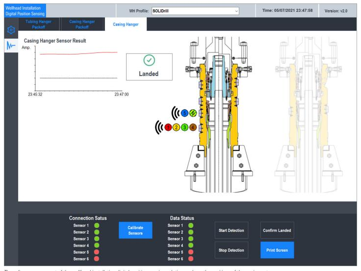
The software component of the wellhead installation digital position sensing solution analyzes the positions of the equipment.
