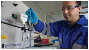
Field-proven, industry-standard Sir Galahad equipment is used to detect mercury content in gas down to 1-ng/m3 concentration levels.
