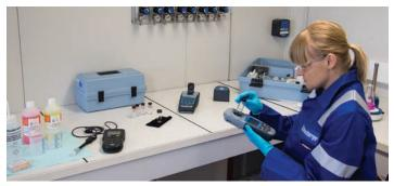
HACH portable laboratory analysis equipment contains rugged field instruments and premeasured reagents for determining key physical and chemical properties of water.
