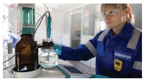
Automatic titration following ASTM International UOP 212 procedures allows for faster, more reliable analysis of sulfur compounds.
