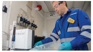
The fully portable MicroGC with an integrated thermal conductivity detector enables quick and accurate measurement of  $C_1$ - $C_2$  hydrocarbons,  $CO_2$ ,  $N_2$ , and  $H_2S$  down to 50 ppm.
